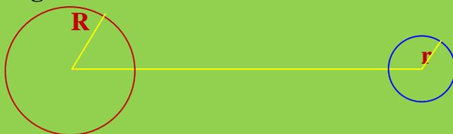
$$V_1 = K \cdot q_1 / R_1 ; q_1 = V_1 \cdot R_1 / K ;$$
