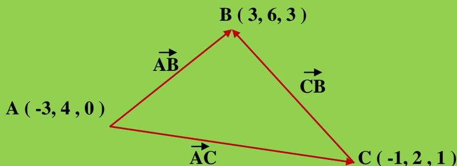
$$\begin{aligned}\vec{AB} & [ (3 - (-3)), (6 - 4), (3 - 0) ] \rightarrow \vec{AB} (6, 2, 3) \\ \vec{AC} & [ (-1 - (-3)), (2 - 4), (1 - 0) ] \rightarrow \vec{AC} (2, -2, 1) \\ \vec{CB} & [ (3 - (-1)), (6 - 2), (3 - 1) ] \rightarrow \vec{CB} (4, 4, 2)\end{aligned}$$
